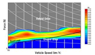
Figure 12: Comparison of fuel consumption of "Hybrid Drive" and "Engine Drive"
