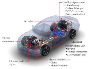
Figure 9: Overall system configuration of 2014 Honda Accord Plug-In
