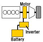
Figure 2: Parallel hybrid electric vehicle (Honda IMA)
