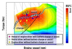
Figure 16: Engine operating point
