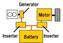
Figure 1: Series hybrid electric vehicle
