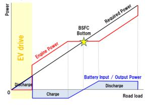
Figure 20: Schematic drawing of basic power management
