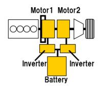
Figure 3: Series-parallel Hybrid (Toyota THS)
