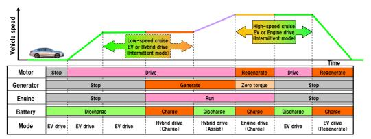
Figure 11: Driving mode transition of typical driving cycle
