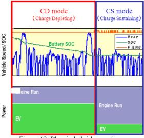
Figure 13: Plug-in hybrid operation
