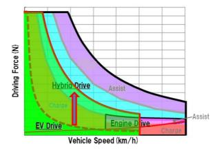
Figure 15: Operation areas of three driving modes (Charge Depleting mode)
