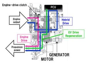
Figure 10: Power flow of e-CVT
