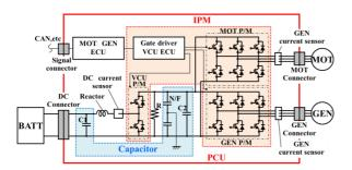
Figure 8: Block diagram of PCU
