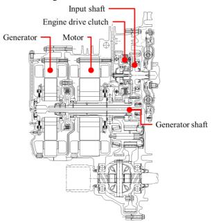
Figure 6: Cross-sectional view of e-CVT
