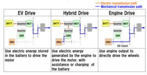
An outline of mode transition in a typical driving cycle is shown in Figure 11. During low-load situation such as launching or city driving, "EV Drive" is mainly selected. Then, the driving mode is switched to "Hybrid Drive" for the acceleration during normal-load or heavy-load situation.
