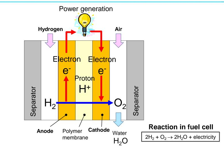
Extracts electrons by reacting hydrogen and oxygen to generate electricity (opposite of water electrolysis)
