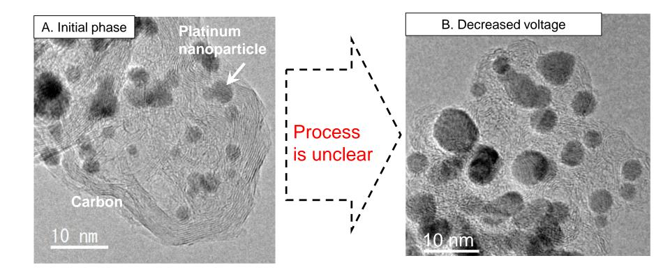
The process of platinum nanoparticle coarsening cannot be fully understood using conventional techniques
