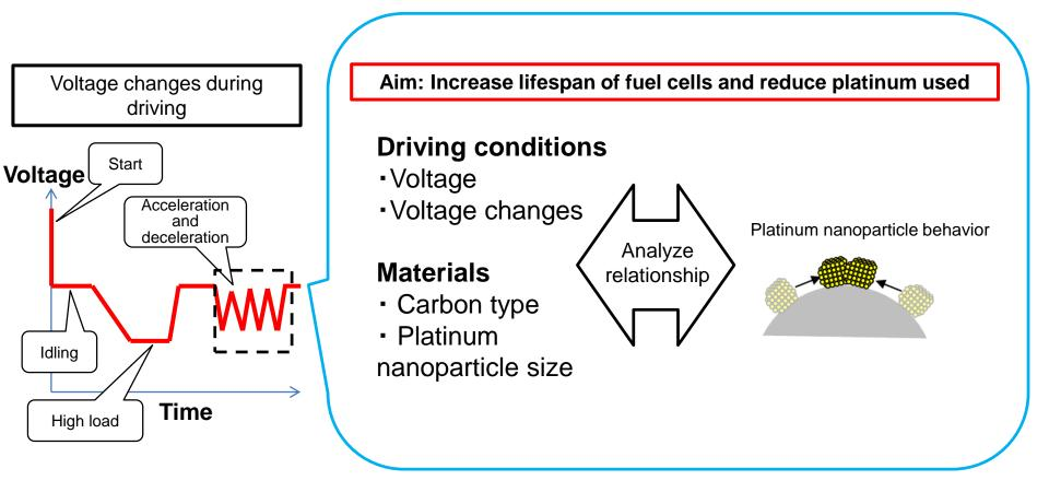
Analysis of relationship between voltage changes during driving and platinum nanoparticle behavior changes
