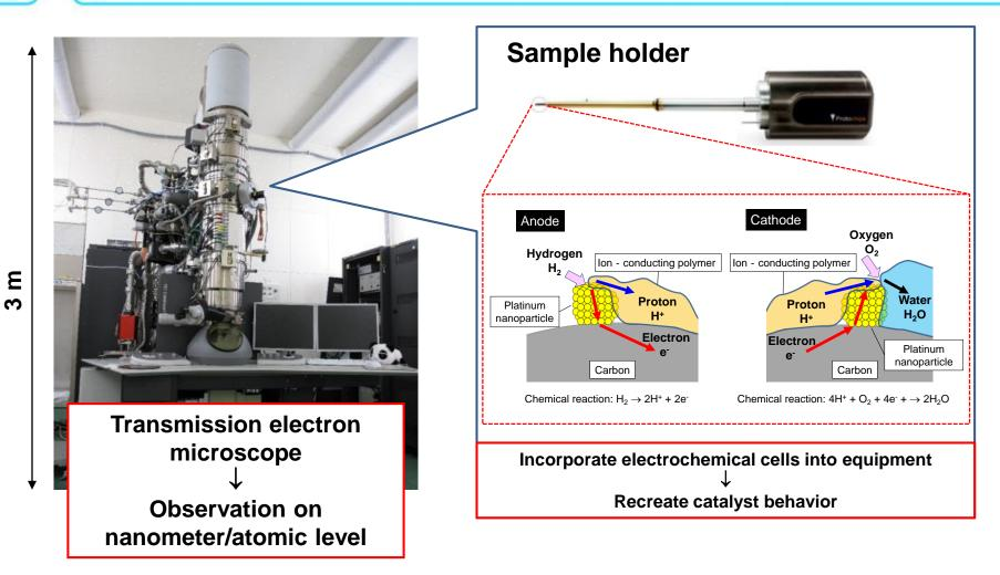
Recreate a fuel cell catalyst chemical reaction in a transmission electron microscope
