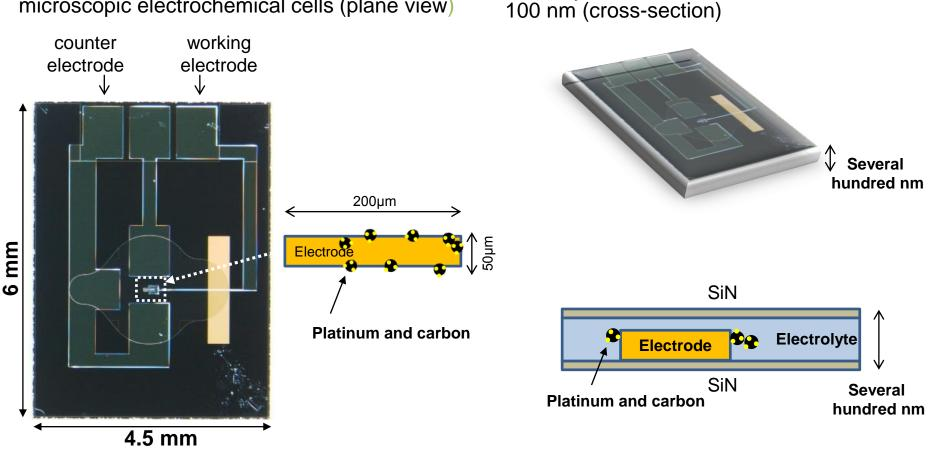
Using micro-electromechanical systems technology to create microscopic electrochemical cells that can be observed via transmission electron microscope
