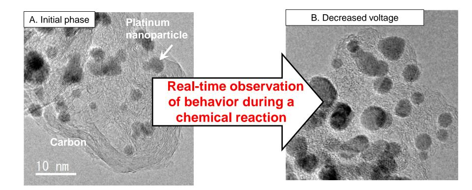
Aim: identify behavior, conditions and materials that make platinum nanoparticles prone to coarsening
