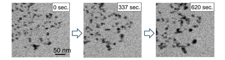
Successful real-time observation of platinum nanoparticle behavior at nanometer levels during a chemical reaction leading to coarsening
