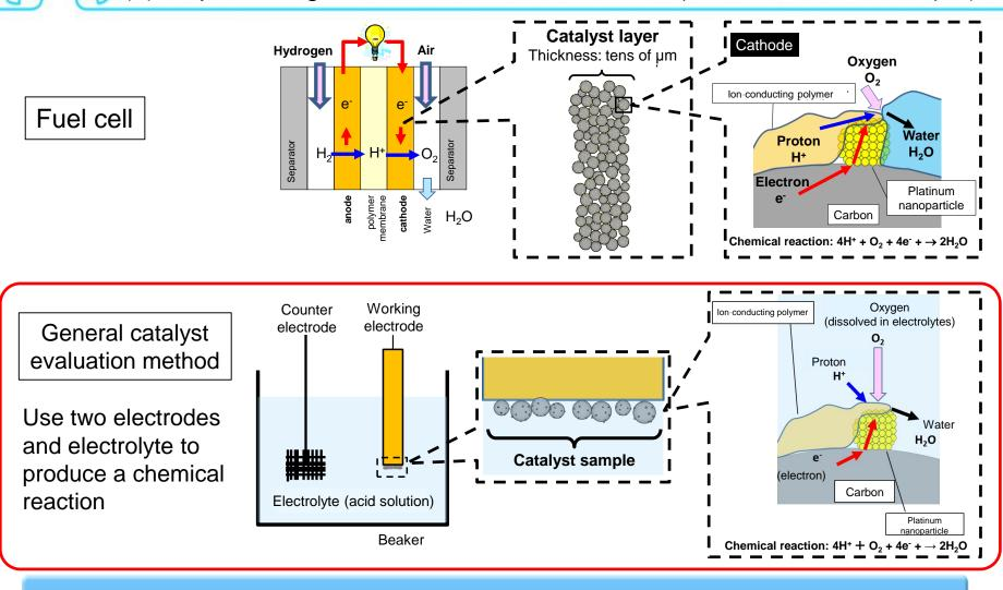
The conventional technique uses the general catalyst evaluation method to reproduce the chemical reactions that occur in fuel cells
