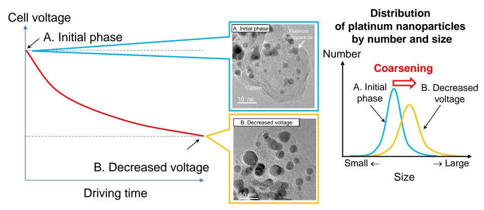
Conventional technology compares platinum nanoparticle size during the initial phase and after voltage is decreased
