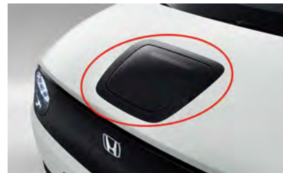
Charge port in the hood
