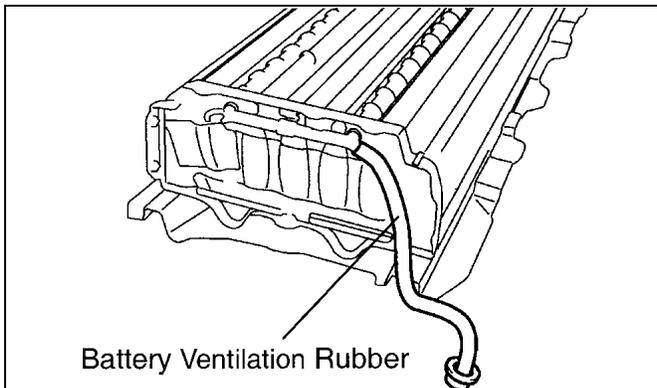
**3. REINSERT THE BATTERY VENTILATION HOSE INTO THE VEHICLE**
