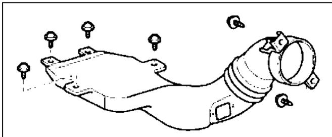
**4. REINSTALL THE QUARTER VENTILATOR DUCT**
