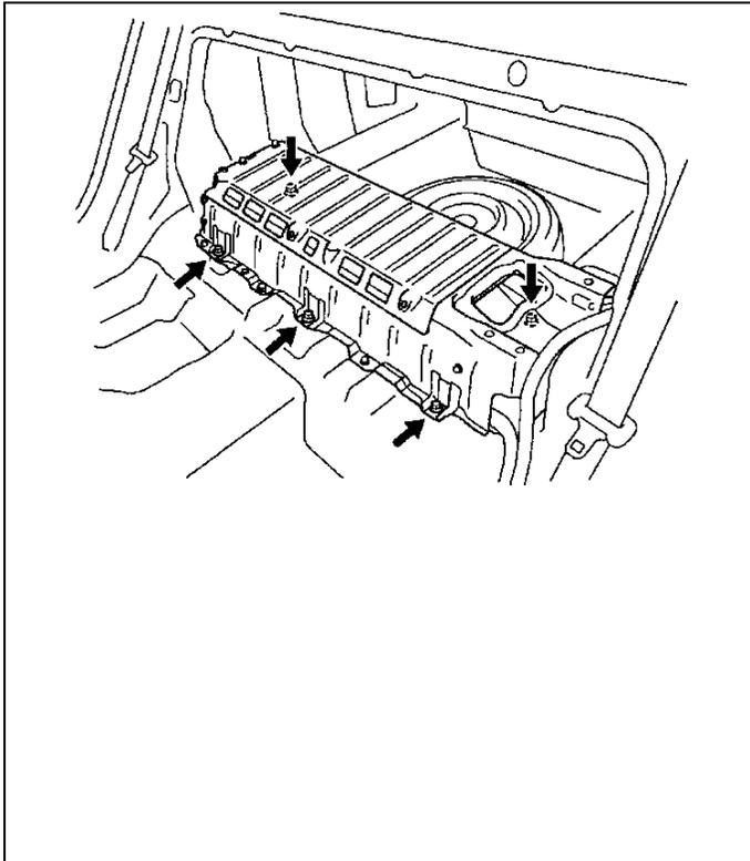
(b) Remove the 5 bolts and the HV battery.
