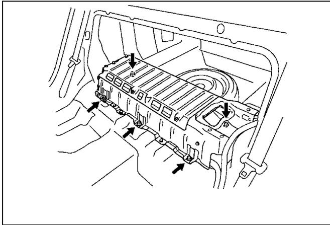
(d) Reinstall and tighten the 5 bolts for the HV battery.
